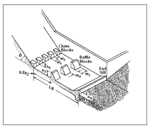
Figure 8.3. USBR Type III Stilling Basin
