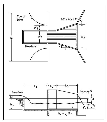
Figure 11.4. Box Inlet Drop Structure
