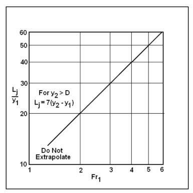
Figure 6.8. Jump Length Circular Channel with  $y_2 < D$
