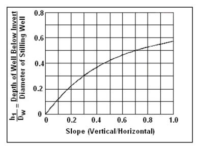
Figure 12.3. Depth of Stilling Well Below Invert (USACE, 1963)
