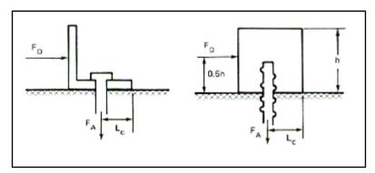
Figure C.1. Forces Acting on a Roughness Element
