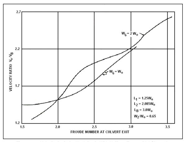
Figure 9.12. Velocity Ratio for Hook Basin With Uniform Trapezoidal Channel
