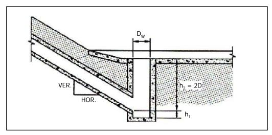
Figure 12.1. US Army Corps of Engineers' Stilling Well (USACE, 1963)
