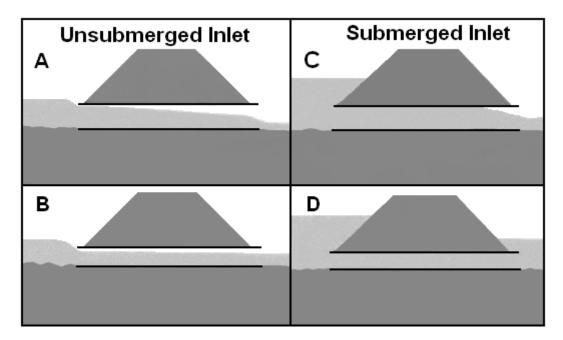
Figure 3.1. Outlet Control Flow Types
