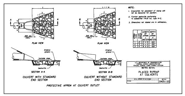
Figure 10.4. Placed Riprap at Culverts (Central Federal Lands Highway Division)
