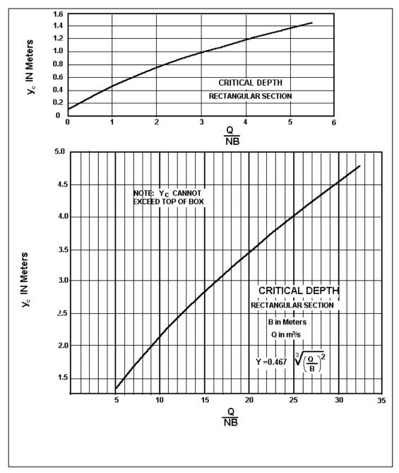
Figure B.1 (SI). Critical Depth Rectangular Section (Normann, et al., 2001)
