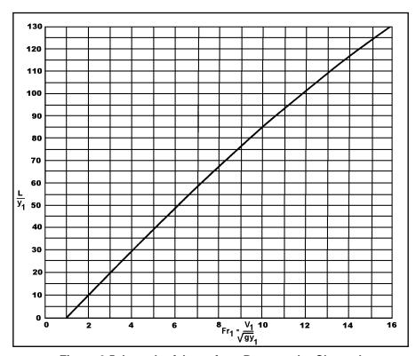
Figure 6.5. Length of Jump for a Rectangular Channel
