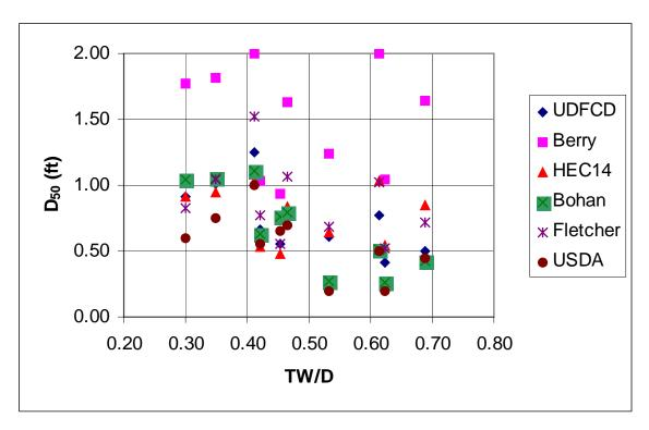
Figure D.3.  $D_{50}$  versus Relative Tailwater Depth
