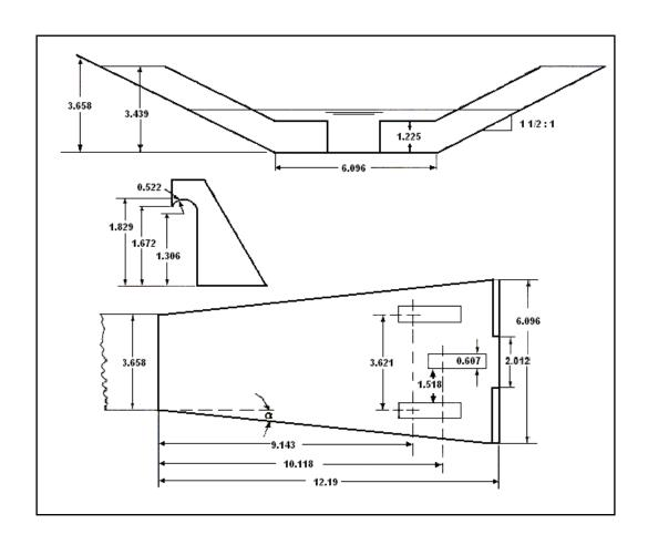
Sketch for the Hook Basin with Warped Wingwalls Design Example (SI)
