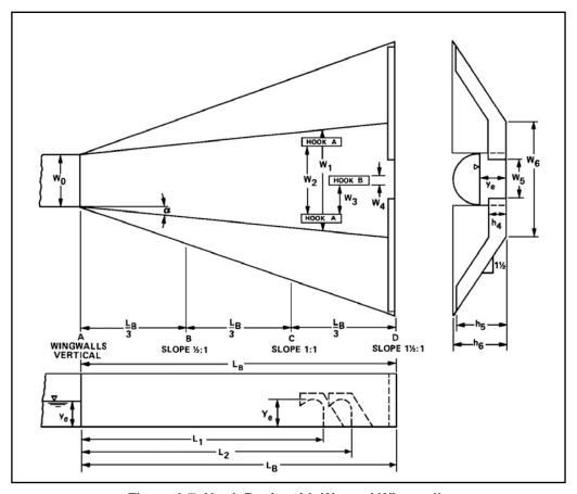
Figure 9.7. Hook Basin with Warped Wingwalls
