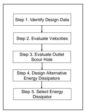
Figure 1.1. Energy Dissipator Design Procedure
