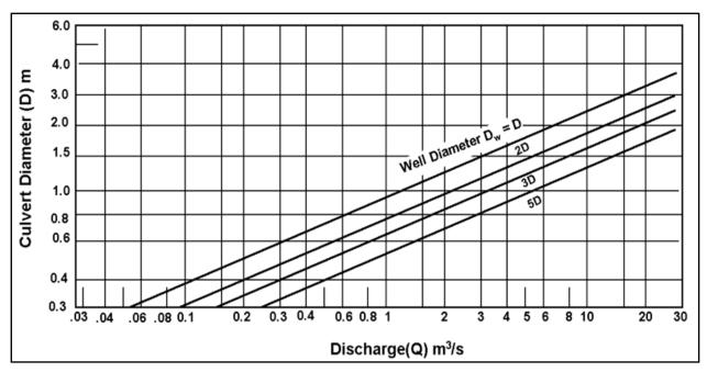
Figure 12.2 (SI). Stilling Well Diameter, D<sub>W</sub> (USACE, 1963)
