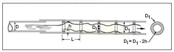
Figure 7.4. Definition Sketch for Tumbling Flow in Circular Culverts
