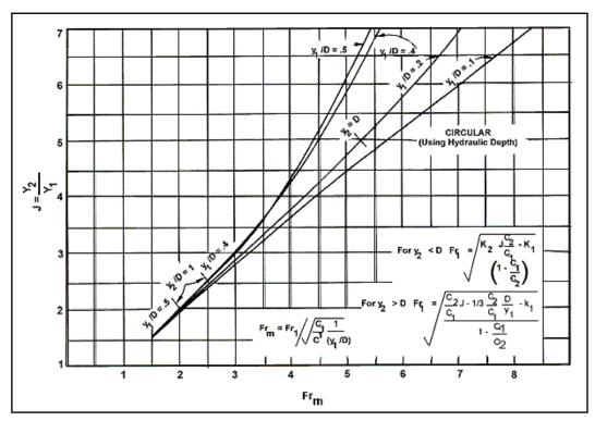
Figure 6.7. Hydraulic Jump - Horizontal, Circular Channel (hydraulic depth)
