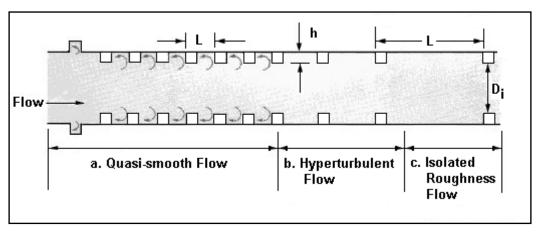
Figure 7.6. Flow Regimes in Rough Pipes
