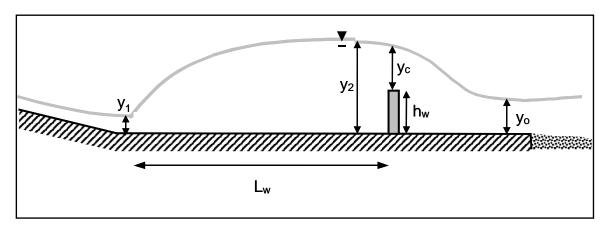
Figure 7.11. Weir Placed near Outlet of Box Culvert
