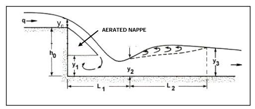
Figure 11.1. Flow Geometry of a Straight Drop Spillway
