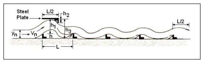
Figure 7.2a. Tumbling Flow in a Box Culvert or Open Chute: Recommended Configuration
