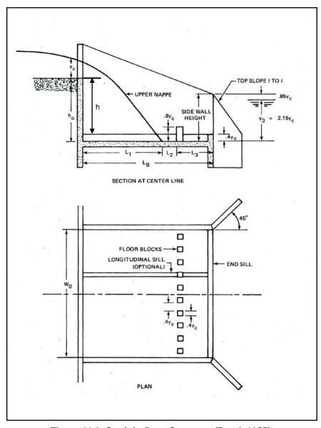
Figure 11.3. Straight Drop Structure (Rand, 1955)
