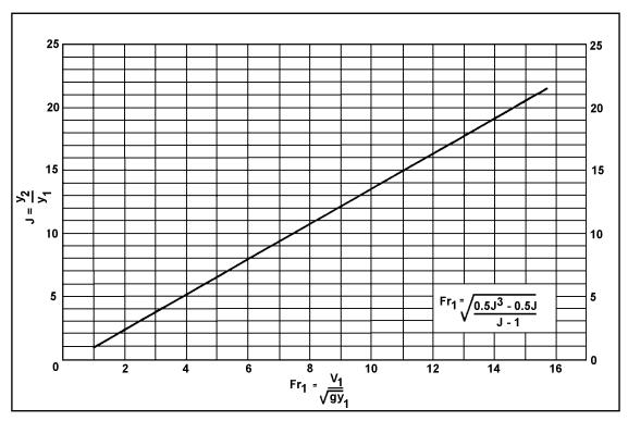
Figure 6.4. Hydraulic Jump - Horizontal, Rectangular Channel
