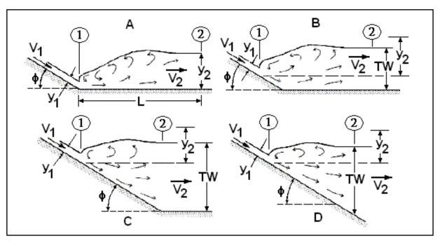
Figure 6.10. Hydraulic Jump Types Sloping Channels (Bradley, 1961)
