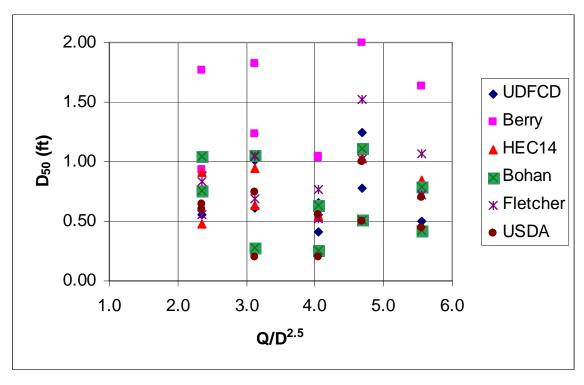
Figure D.2. D<sub>50</sub> versus Discharge Intensity
