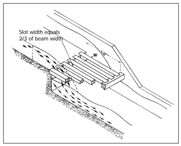
Figure 11.2. Drop Structure with Grate
