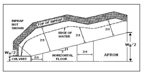
Figure 10.2. Half Plan of Riprap Basin
