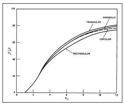
Figure 6.9. Relative Energy Loss for Various Channel Shapes
