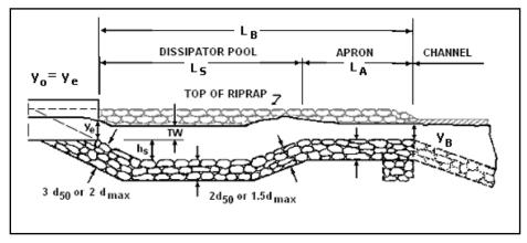
Figure 10.1. Profile of Riprap Basin
