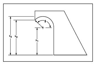
Figure 9.11. Hook for Uniform Trapezoidal Channel Basin
