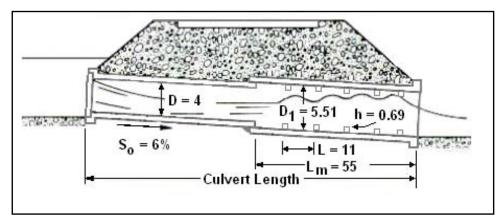
Solution for Tumbling Flow Example for a Circular Culvert (CU)
