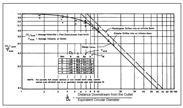
Figure 10.3. Distribution of Centerline Velocity for Flow from Submerged Outlets
