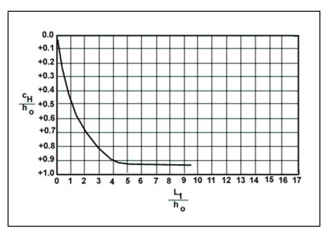
Figure 11.10. Relative Head Correction for  $h_0/W_2 \ge 1/4$  with Control at Headwall Opening
