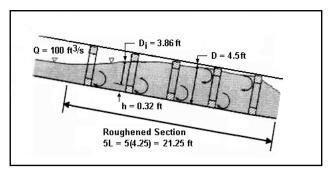
Sketch for Increased Resistance In a Circular Culvert Design Example (CU)
