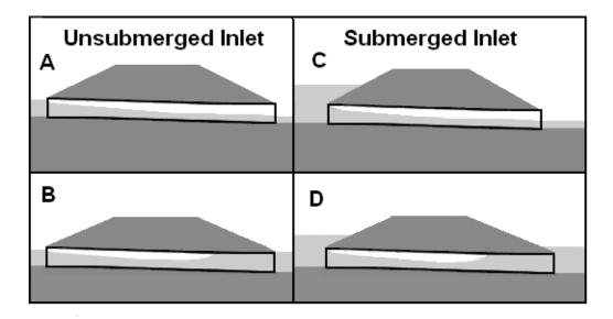
Figure 3.5. Inlet Control Flow Types
