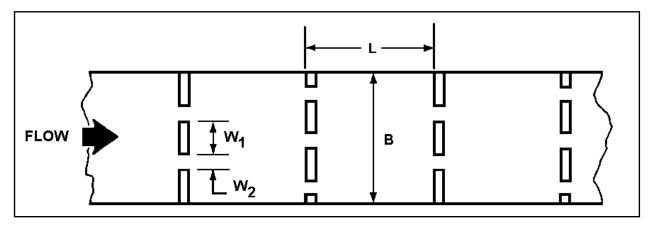
Figure 7.3. Definition Sketch for Slotted Roughness Elements
