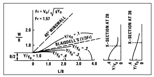
Figure 4.2. Dimensionless Water Surface Contours (Watts, 1968)
