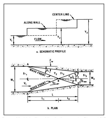
Figure 4.6. Supercritical Inlet Transition for Rectangular Channel (USACE, 1994)
