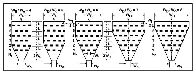
Figure 9.3. Roughness Configurations Tested
