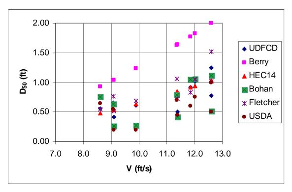
Figure D.1. D<sub>50</sub> versus Outlet Velocity
