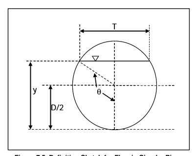
Figure 7.5. Definition Sketch for Flow in Circular Pipes
