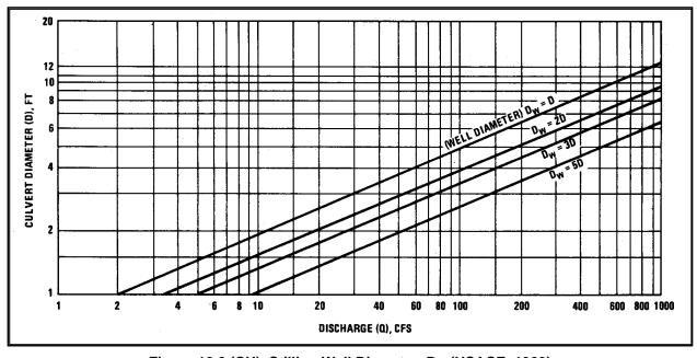
Figure 12.2 (CU). Stilling Well Diameter, D<sub>W</sub> (USACE, 1963)
