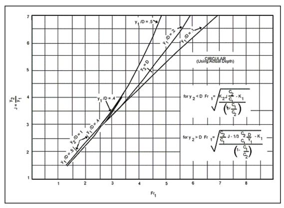
Figure 6.6. Hydraulic Jump - Horizontal, Circular Channel (actual depth)
