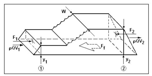
Figure 6.3. Hydraulic Jump in a Horizontal Channel
