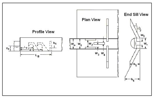
Figure 9.10. Hook Basin with Uniform Trapezoidal Channel
