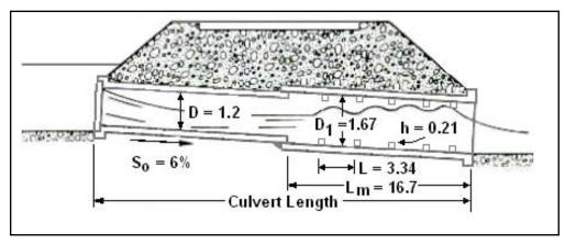
Solution for Tumbling Flow Example for a Circular Culvert (SI)
